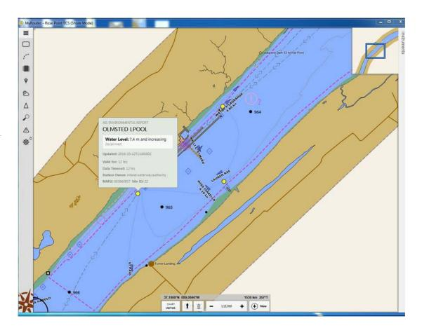
A commercial electronic chart system shows both electronic Aids to Navigation (eATON) and enhanced Marine Safety Information (eMSI) being broadcast in the vicinity of Olmsted Lock. The blue diamonds are eATONs that assist the mariner in navigating around the lock. The yellow dots are eMSI, which provide the mariner critical pieces of information that enhance situational awareness; the eMSI broadcast selected displays the current water level at that location.
