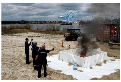
Smaller-scale freshwater insitu test burns in progress with research and fire safety team.
