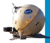
Using ground antennas. like the one shown here. Coast Guard researchers explored deployable satellite communications.
